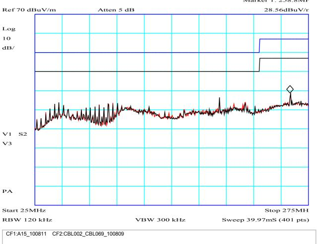
PLOT 2 Radiated Emissions - 25MHz to 275MHz - Vertical Polarisation - Laptop PC with and without two radiation harmoniser chips fitted
