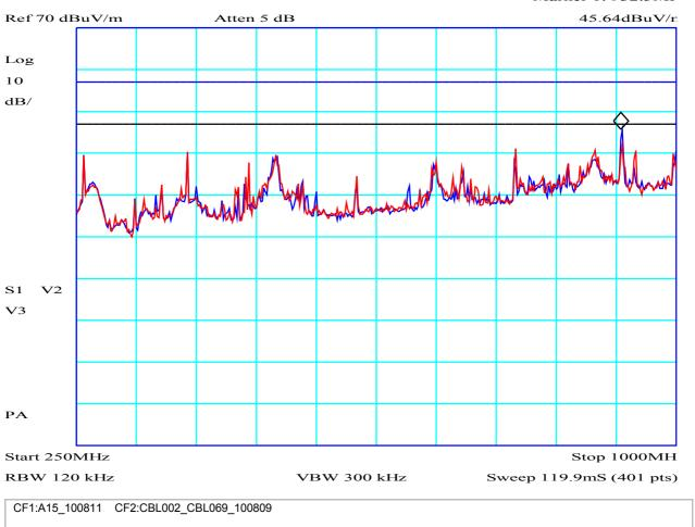
PLOT 4 Radiated Emissions - 250MHz to 1GHz - Horizontal Polarisation - Laptop PC with and without two radiation harmoniser chips fitted
